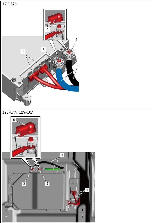
10) Remove the bolts (1), and then remove the lithium-ion battery (2).
