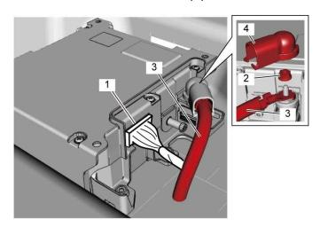
7) Remove the bolts (1), and then remove the lithium-ion battery (2).
