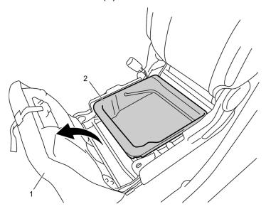
4) Remove the cover (1) and the rear duct (2) Litium-ion battery 12V 36Wh
