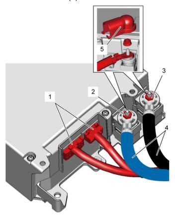
7) Remove the bolts (1), and then remove the lithium-ion battery (2).
