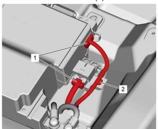
6) Remove the positive terminal nuts (2) under the terminal covers (1), and then remove the cables (3).
