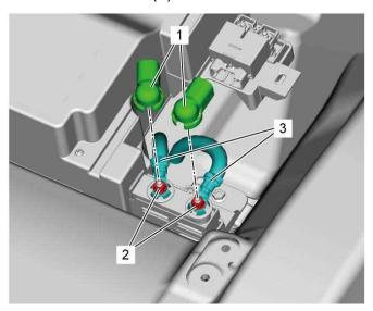
7) Remove the bolts (1), and then remove the lithium-ion battery (2).
