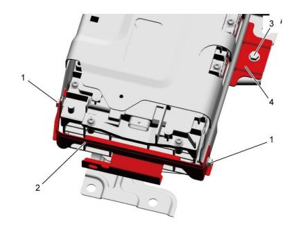
17) Remove the lithium-ion battery (1) by pulling it in arrow direction.
