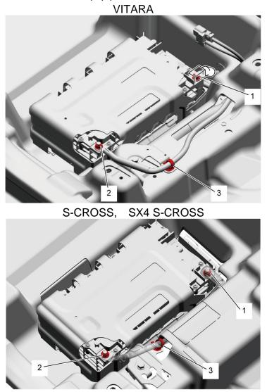
14) Remove the lithium-ion battery holder bolts (1), and then remove the lithium-ion battery holder (2) and the lithium-ion battery (3).
