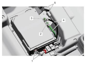
11) Remove the bolts (1), and then remove the lithium-ion battery (2).
