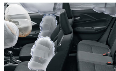
Image of car interior during airbag deployment (model: Swift)
