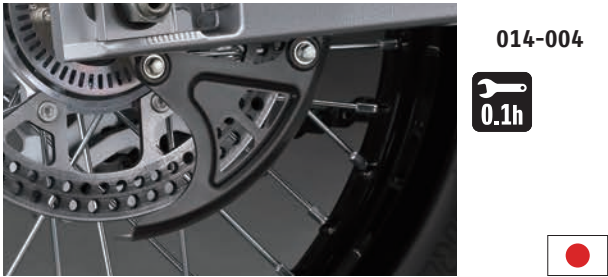
Rear Brake Disc Cover 69230-37810-000 Reduces the adherence of mud to the brake disc.
