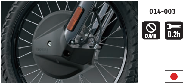
Front Brake Disc Cover 59230-37810-000 Reduces the adherence of mud to the brake disc. Not applicable for DR-Z4SM. *Not in combination with Front Axle Slider (p/n 54700-37810-000).
