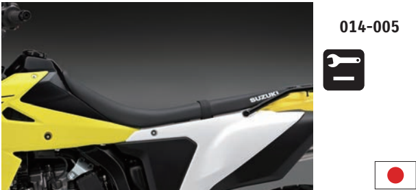
Low Seat 45100-37810-C1U 30mm lower than the standard seat. It uses a higher density polyurethane foam to enhance ride comfort while ensuring good foot reach.
