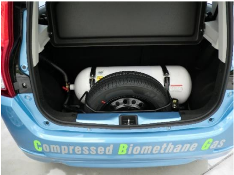
CNG Tank in the Wagon R trunk
