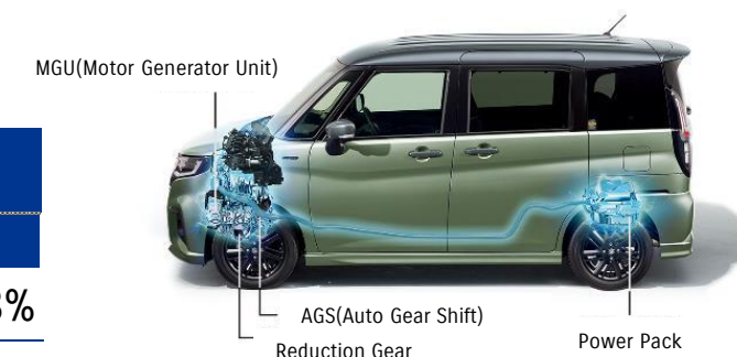
Mild hybrid system (HYBRID)
