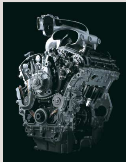
The new GM-designed global V6 engine will go onto XL7
