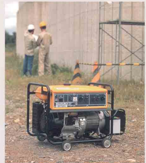
Generator SV7500E powered with V420 4-stroke OHV engine
