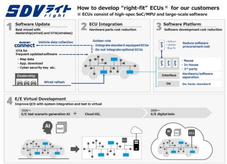
Note) The Cloud HIL of "E/E Virtual Development" in the above diagram is the task which will be conducted at the SUZUKI-TATA ELXSI Cloud HIL Center.
