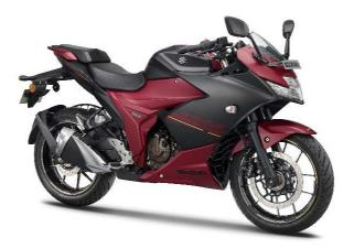
GIXXER SF 250 is a 250cc road sports bike equipped with Suzuki's original oil-cooled engine. The new specification which applies to bioethanol up to 85% has been added. By improving the fuel injector, fuel pump, and fuel filter, users can use wide range of bio-ethanol fuel. Because bio-ethanol fuel derives from plants, it contributes to the reduction of CO<sub>2</sub> compared to the conventional fossil fuel.
