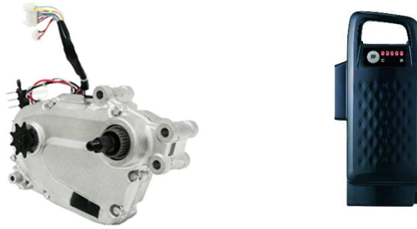
Drive unit and battery of Panasonic Cycle Technology's e-bike
