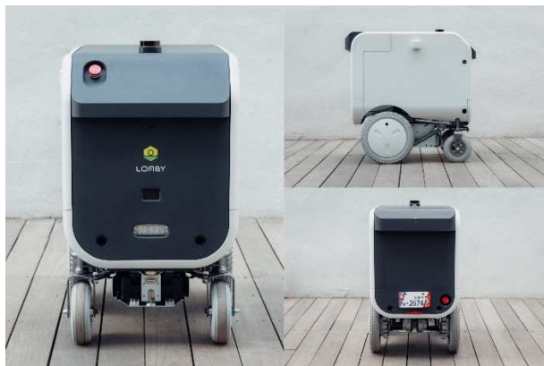
Prototype of autonomous delivery robot using a base of electric wheelchair
