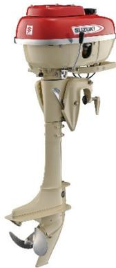
D55 (Suzuki's first outboard motor)
