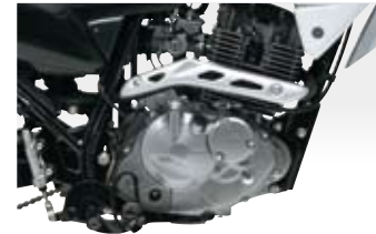
Fuel-injected 125cm 3 engine
