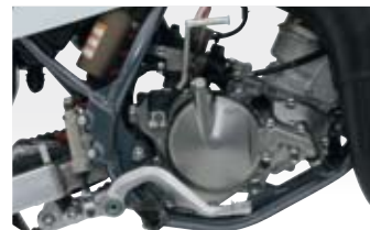
84.7cm 3 2-stroke engine
