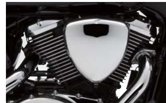
Liquid-cooled 45-degree V-Twin engine
