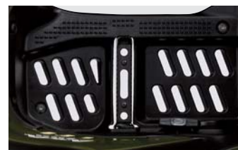
(Dummy) Full floorboards with drain holes
