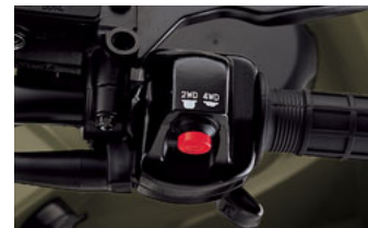
Mode selection switch for 2WD and 4WD
