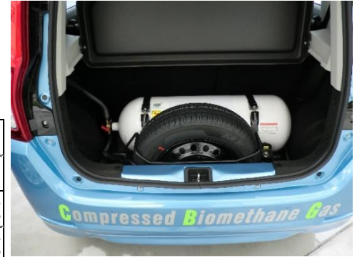
CNG Tank in the Wagon R trunk
