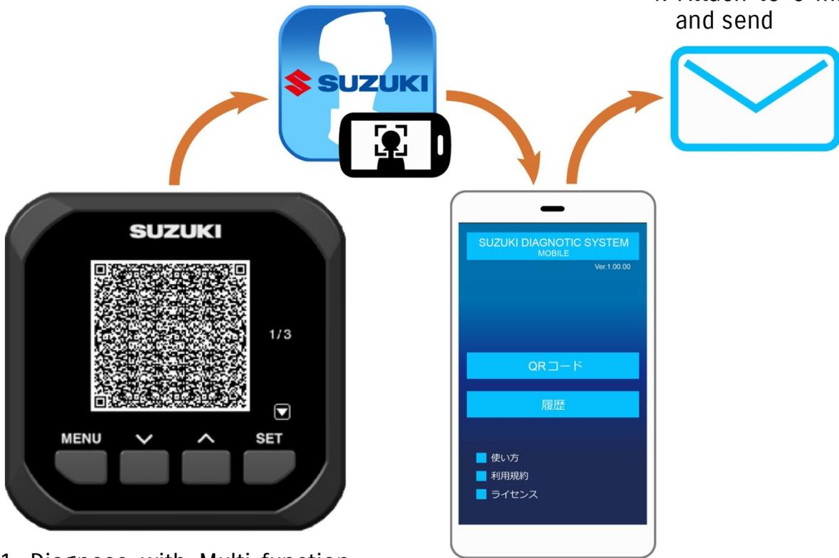
1. Diagnose with Multi-function Gauge and display engine information as QR Codes
