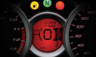
Engine mode indicator (The photo is edited to show all of the instrument lights and displays)
