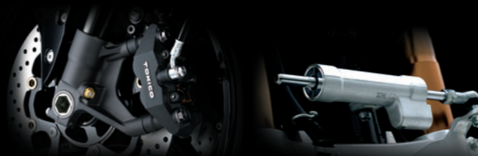
Radial-mount TOKICO front brake caliper
