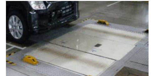
(2) Side slip inspection
