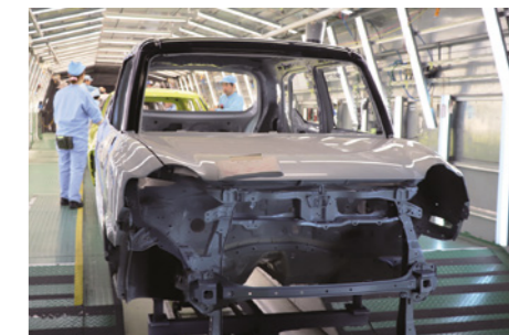
塗装(塗装検査) Painting (Painting Inspection)
