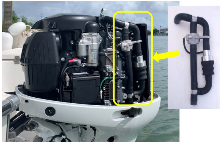
Outboard motor installed with Micro-Plastic Collecting Device
