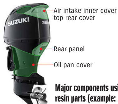
Adopted pre-colored recycled PP resinous materials for 14 exterior resin parts
