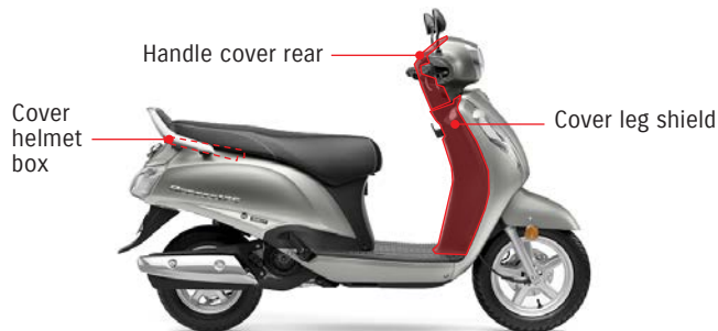
Adopted pre-colored recycled PP resinous materials for 3 exterior resin parts
