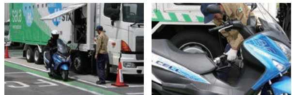
Hydrogen filling at Hamamatsu Hydrogen station (mobile) (Actual operation started in March 2017)
