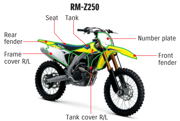
PP materials were adopted for 8 parts which cover 80% of exterior resin and seat bottom plate
