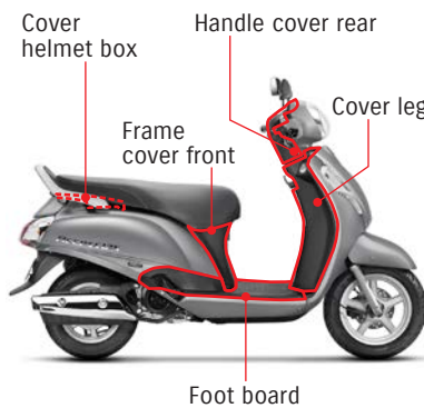
PP materials were adopted for 5 exterior resin parts
