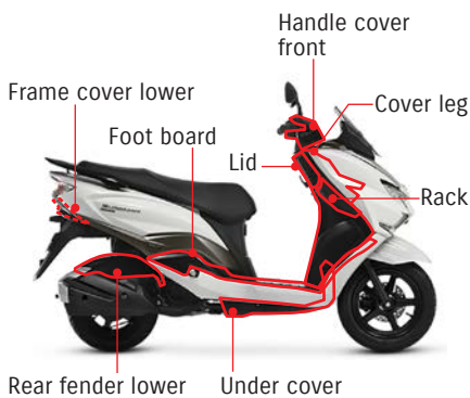
PP materials were adopted for 8 exterior resin parts
