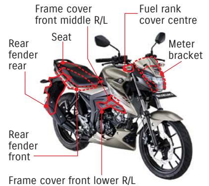
PP materials were adopted for 7 exterior resin parts and seat bottom plate
