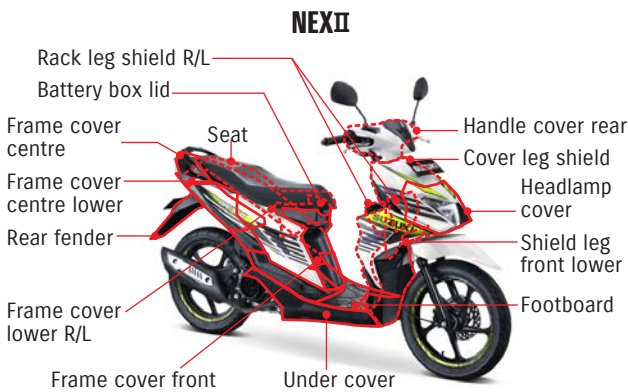
PP materials were adopted for 15 exterior resin parts and seat bottom plate
