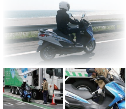
Hydrogen filling at Hamamatsu Hydrogen station (mobile) (Actual operation started in March 2017)
