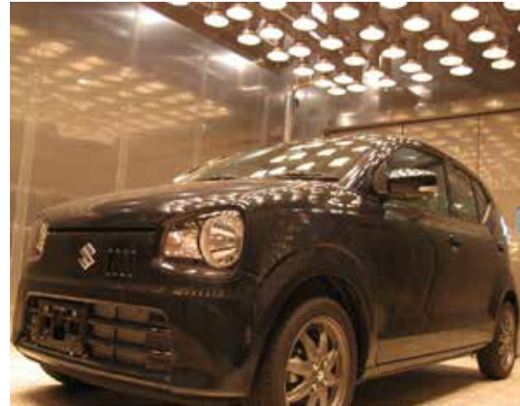
Cabin VOC measurement in a newly installed constant temperature and humidity testing chamber
