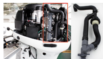
Outboard motor installed with Micro-Plastic Collecting Device
