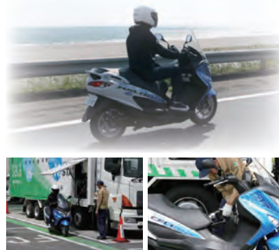
Hydrogen filling at Hamamatsu Hydrogen Station (mobile) (Actual operation started in March 2017)
