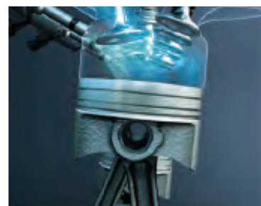
Image of direct-injection in cylinder
