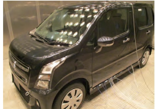
Cabin VOC measurement of the new WagonR Stingray
