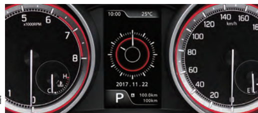
Momentary fuel efficiency, average fuel efficiency, and cruising distance indicators
