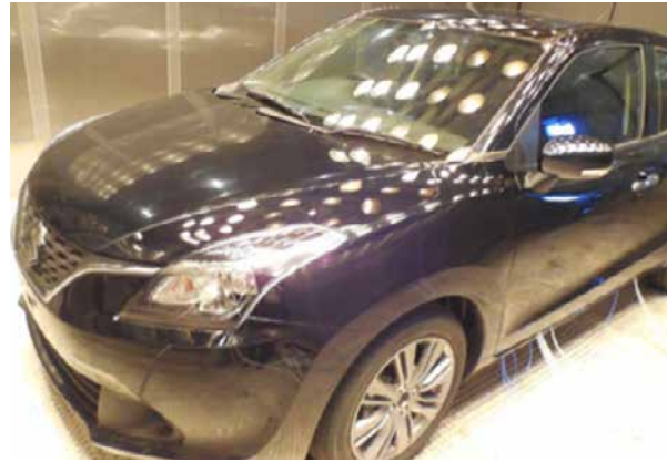
Cabin VOC measurement in a newly installed constant temperature and humidity testing chamber
