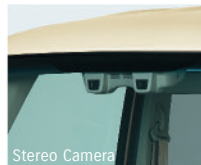
Stereo Camera The stereo cameras are installed in the wiper operating range, so the system works even in the rain. *However, in extremely bad weather (such as heavy rain, snow, fog and the like), it may not work.
