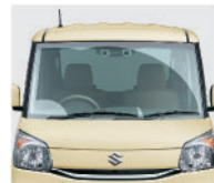
Stereo Camera The stereo cameras are installed in the wiper operating range, so the system works even in the rain. *However, in extremely bad weather (such as heavy rain, snow, fog and the like), it may not work.
