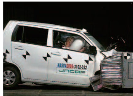
Front offset collision test Source: National Agency for Automotive Safety and Victim's Aid (NASVA)
