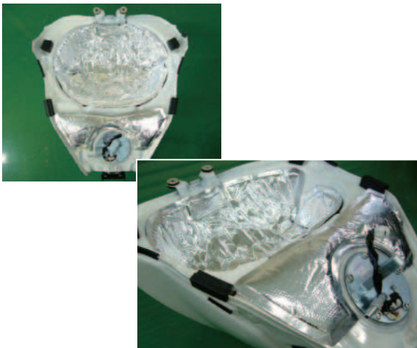
Noise absorbing material (silver sheet) in gasoline tank
